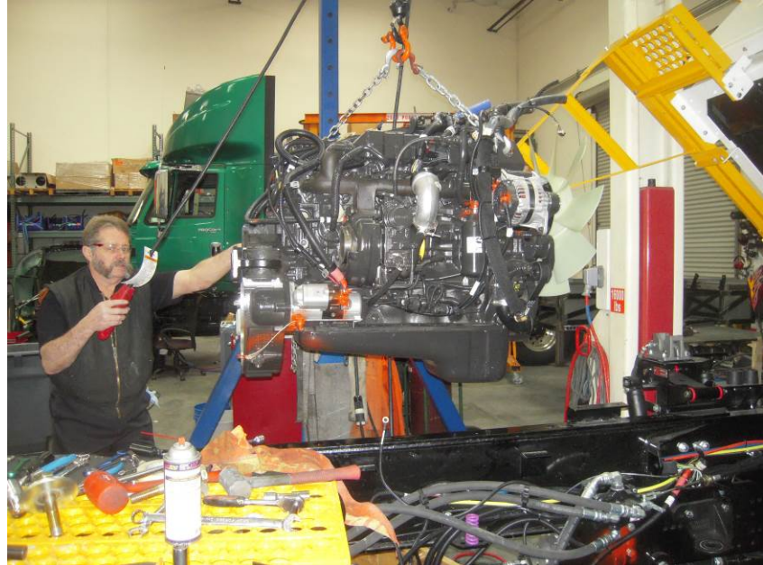
Figure 5. Engine being removed from a Kalmar tractor.
