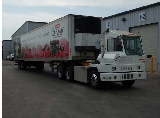
Figure 2. Early prototype electric tractor pulling container at HEB facility in Texas.
