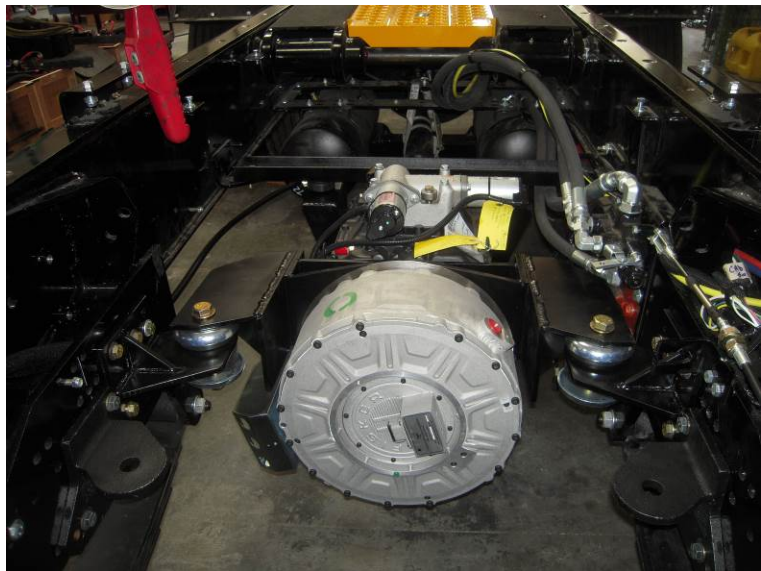
Figure 7. Motive drive subsystem installed.
