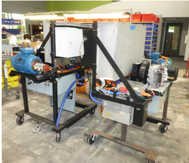
Figure 11. Completed PCAS assemblies prior to tractor installation.
