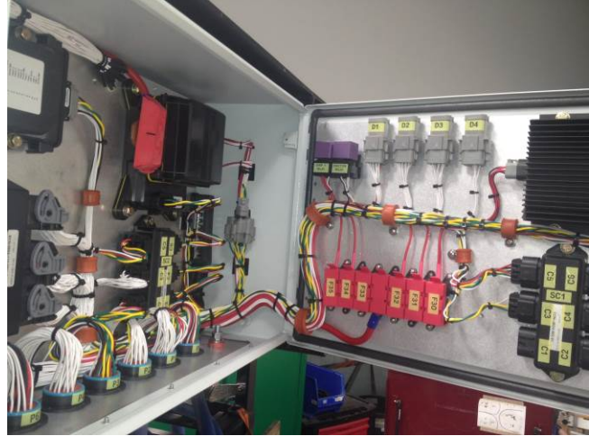
Figure 13. Interior of CCM as integrated into each PCAS assembly.
